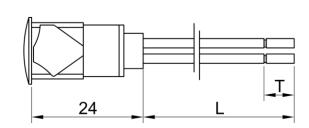
Self-locking LED light indicator with front panel's connection and thin head (thickness 2,5mm)
